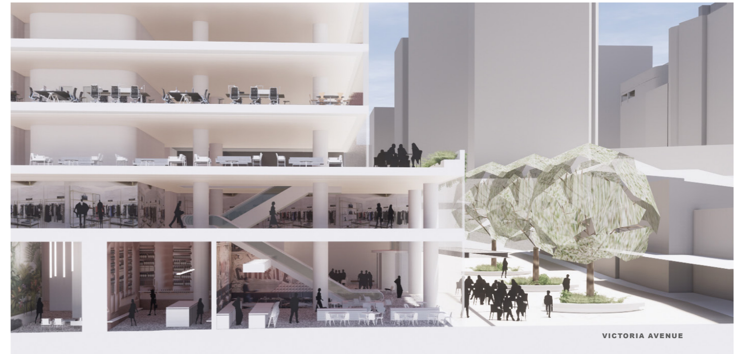
The two storey podium to Victoria Avenue provides the opportunity for clear and accessible vertical circulation to the north-facing rooftop terrace.
